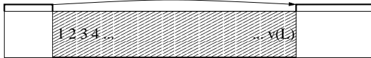
Figure 5. A very good case for mark-split: live data forms one big chunk and marking is consecutive (as shown by the numbers).
